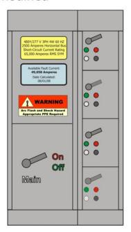
Service equipment in other than dwelling units shall be legibly marked in the field with the maximum available fault current
